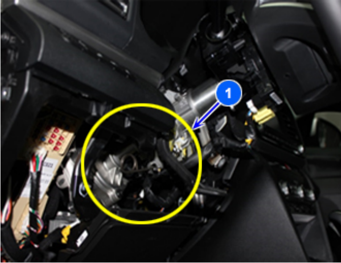
1. MDPS, Steering Angle Sensor - Yaw rate and Lateral Sensor Yaw rate and Lateral Sensor
