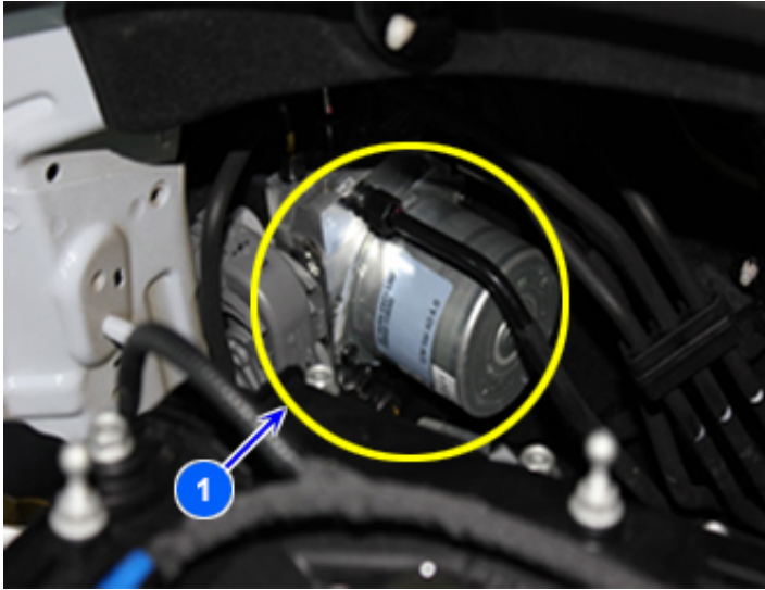
1. ESP(ESC) Control module (ABSCM and Hydraulic Unit) - LKA-L( Lane Keeping Assistance-Line) LKA-L(Lane Keeping Assistance-Line)
