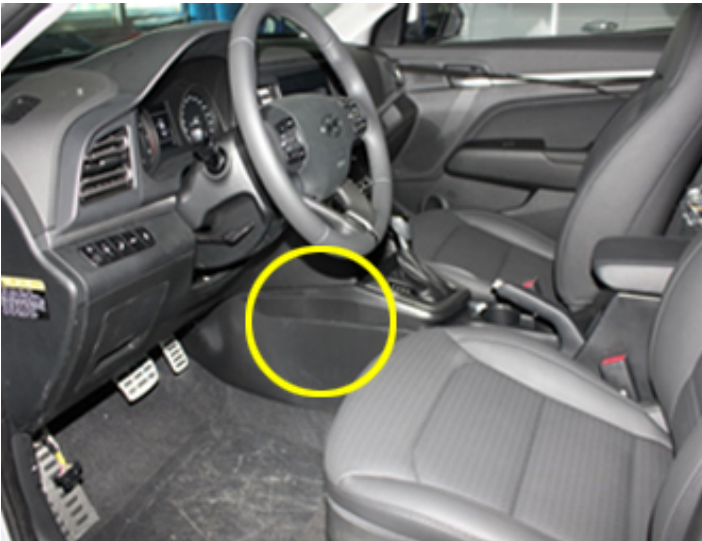
1. SRSCM (Airbag Control Module: Yaw rate and G sensor installed) - ESP(ESC) Control Module ESP(ESC) Control Module
