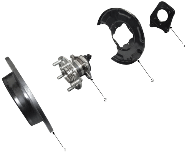
1. Rear brake disc 2. Rear hub bearing 3. Backing plate 4. Bracket [Drum type]
