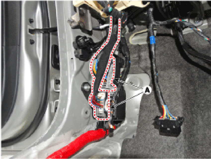
- Disconnect the multi box connectors (A). [Driver's side] [Passenger's side]
