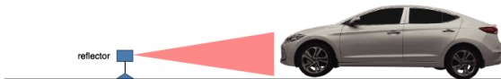
[Leveling: Installation surface of the vehicle and the reflector must be evenly levelled.]
