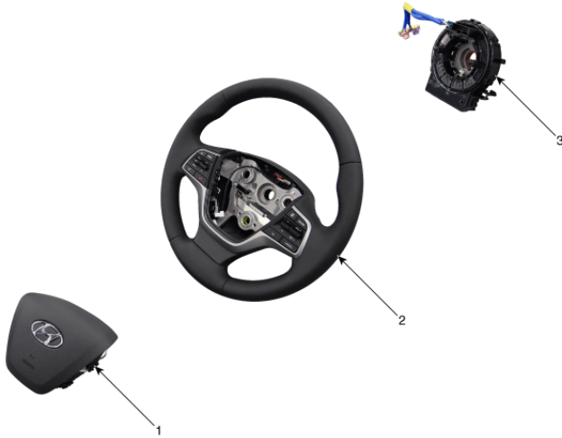
1. Driver Air Bag ( DAB ) 2. Steering Wheel 3. Clock Spring
