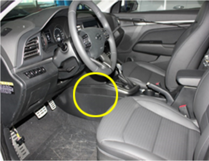
1. Supplemental Restraint System Control Module (SRSCM) - ESP (ECS/TCS) OFF Switch ESP (ECS/TCS) OFF Switch
