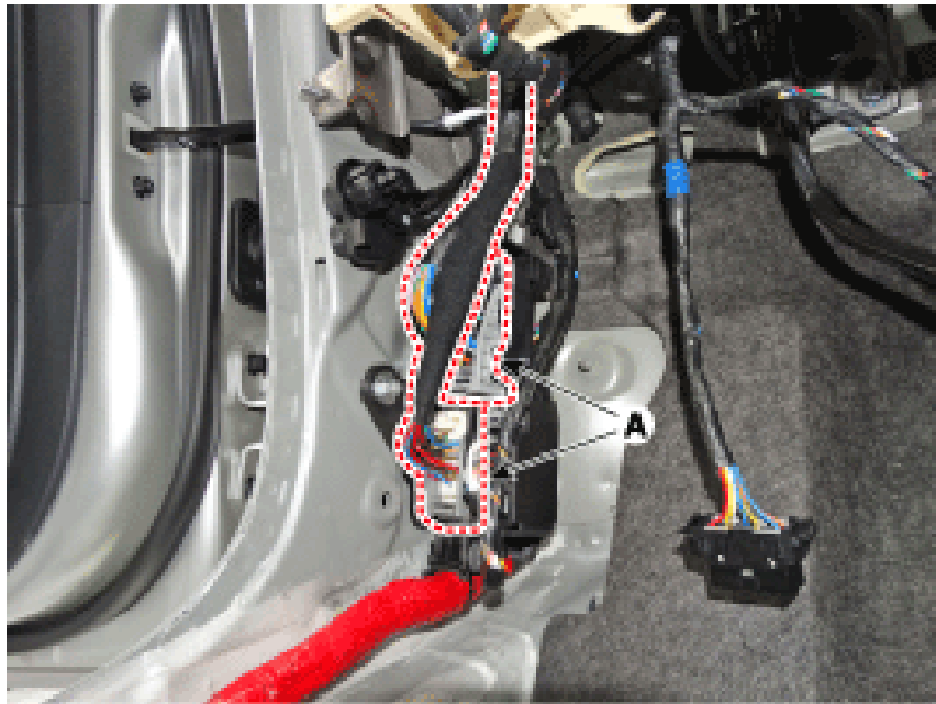
- Disconnect the multi box connectors (A). [Driver's] [Passenger's]
